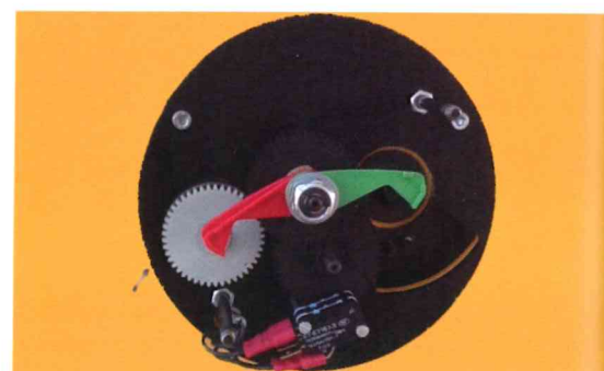
Limit switch very easy to adjust and extremely reliable.
